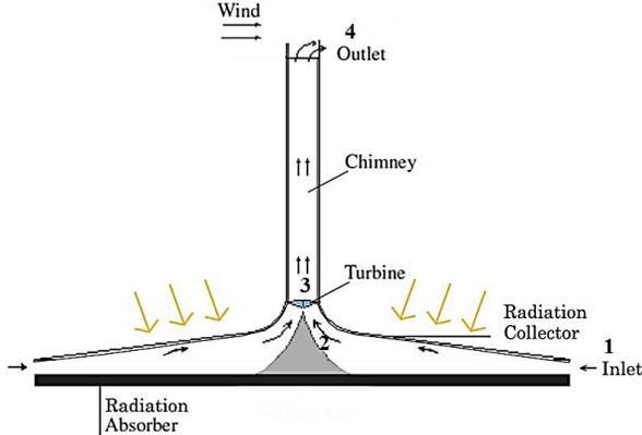
Fig.2. Schematic layout of a solar chimney power plant(Wang et al., 2012)
