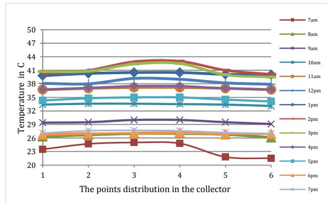
Fig.7. Heat distribution under the collector
