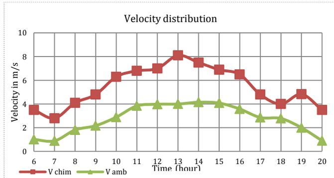
Fig.8. Air velocity of chimney inlet and ambient air velocity
