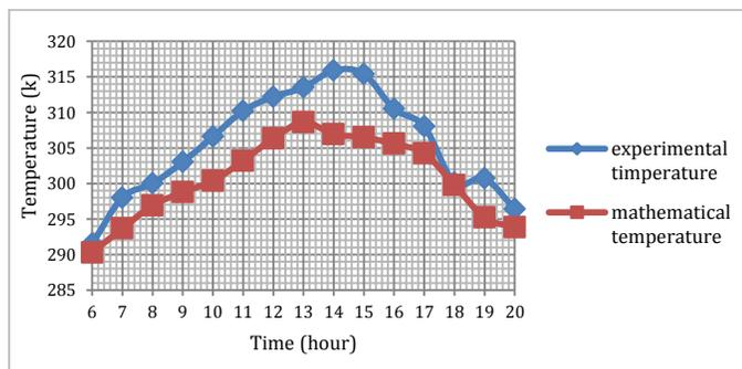
Fig.9. Comparison between the experimental and mathematical model in the chimney inlet temperature value
