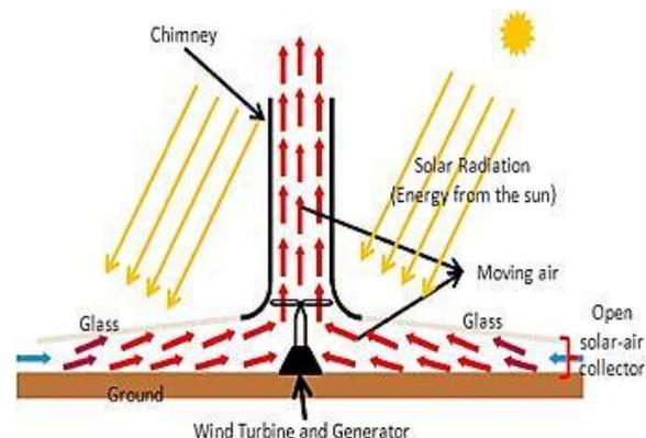
Fig.1. Solar chimney system (Al-Kayiem and Aja, 2016)
