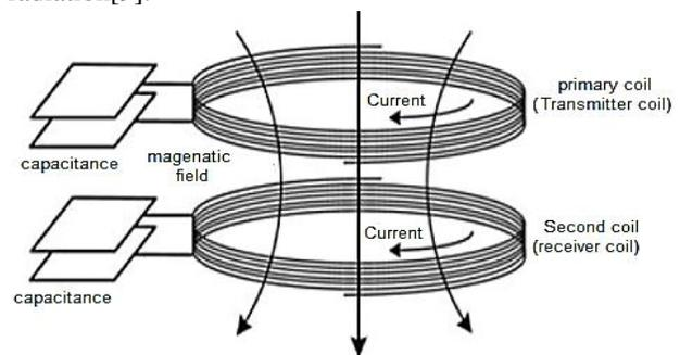
Fig. 2. Resonant inductive coupling
