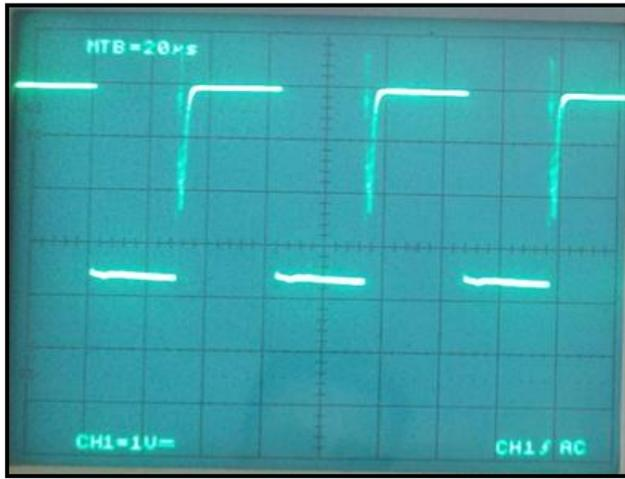
Fig.8. The timer produce square wave with frequency 18.9khz
