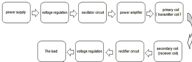
Fig. 5. Block diagram of transmitter and receiver wireless power transfer
