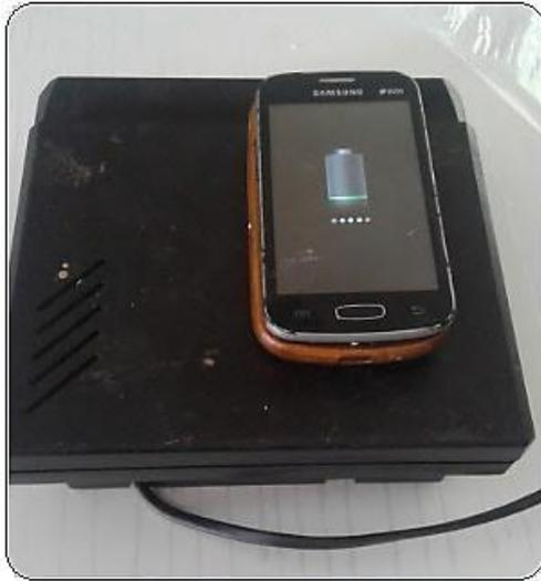
Fig. 12. Prototype of near field WPT
