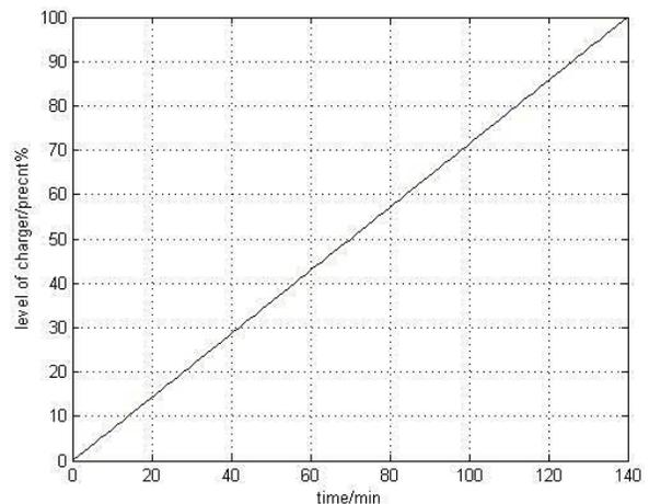
Fig. 11. The relation between time of charge the battery and level of charging
