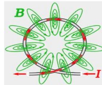
Fig. 6. Current through conductor creates a circular magnetic field
