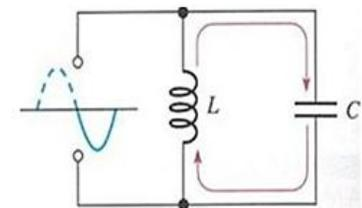
Fig. 4. Tank circuit ( The capacitor discharges as the coil energizes)
