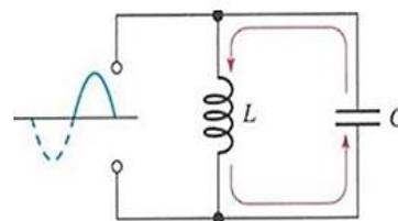
Fig. 3. Tank circuit (The coil de energizes as the capacitor charge)
