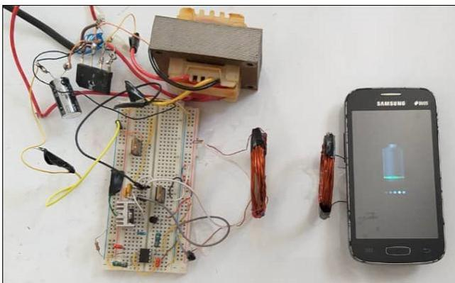
Fig. 9. The practical circuit of WPT in the laboratory
