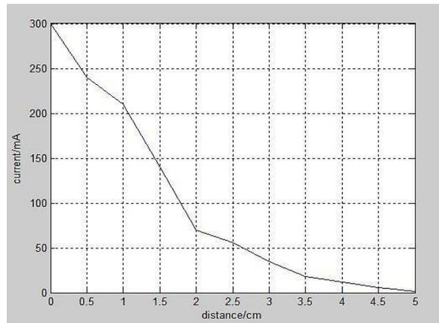
Fig. 10. output current vs. the distance between transmitter and receiver coils
