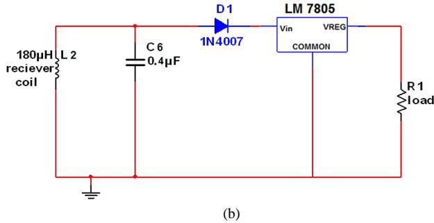
Fig. 7. Implementation of WPT circuit (a)Transmitter circuit (b)Receiver circuit
