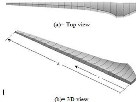
Fig. 2: The geometry of the wind turbine blade.
