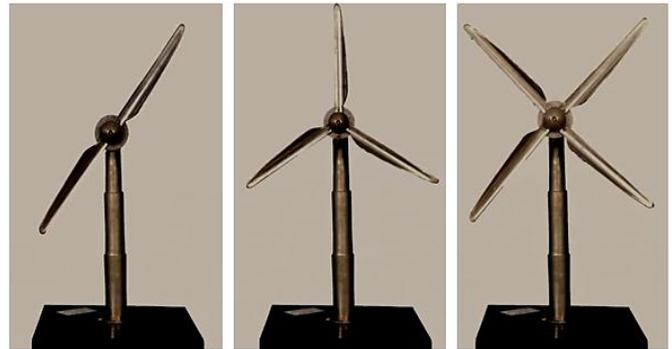
Fig. 1. Three different fabricated small-scale upwind horizontal axis wind turbines for experimental tests: (a) 2-bladed rotor. (b) 3-bladed rotor. (c) 4-bladed rotor.
