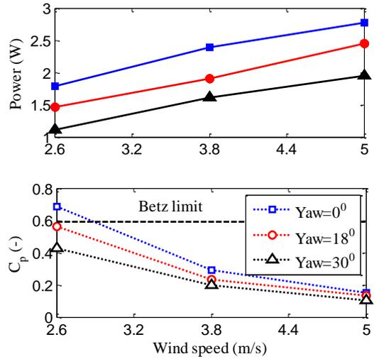
Fig. 6: Performance of the Four-bladed rotor.
