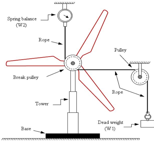
Fig. 3: Rope brake dynamometer to measure torque.
