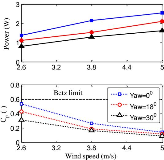
Fig. 4: Performance of the Two-bladed rotor.
