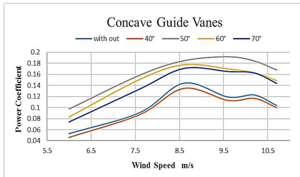
Figure 5. Variation between power coefficient and wind speed with concave guide vanes at different tilt angle.
