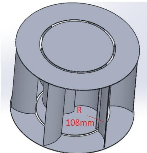
Figure 2. Design of shape concave of guide vane.
