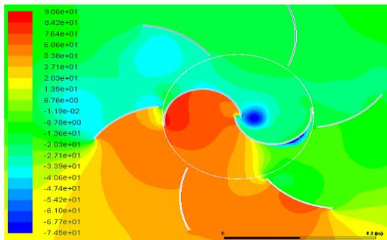
Figure 6. Static pressure Contours for 50° and 10.6 m/s.
