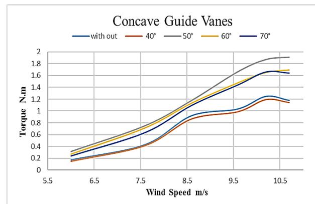
Figure 4. Variation between Torque and wind speed with concave guide vanes at different tilt angle.
