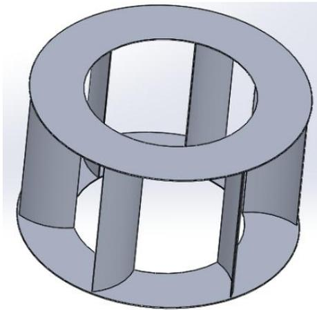
Figure 1. design of guide vane.
