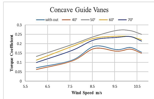
Figure 3. Variation between Torque Coefficient and wind speed with concave guide vanes at different tilt angle.
